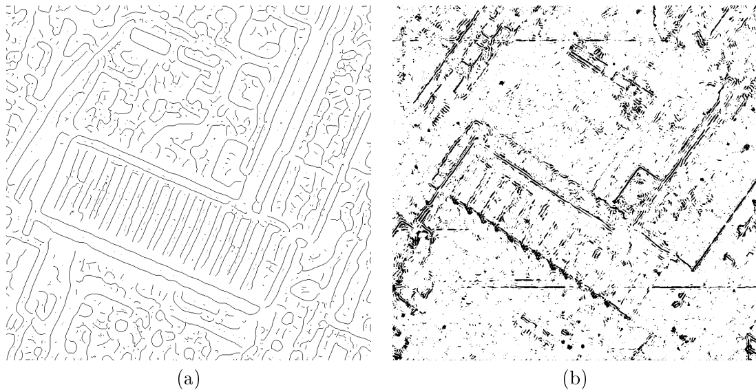
Figure 6.11: (a) Lines extracted with the Canny algorithm applied to the anisotropic diffusion filtered optical image, (b) Lines extracted with the Tupin algorithm applied to the Frost filtered SAR image
